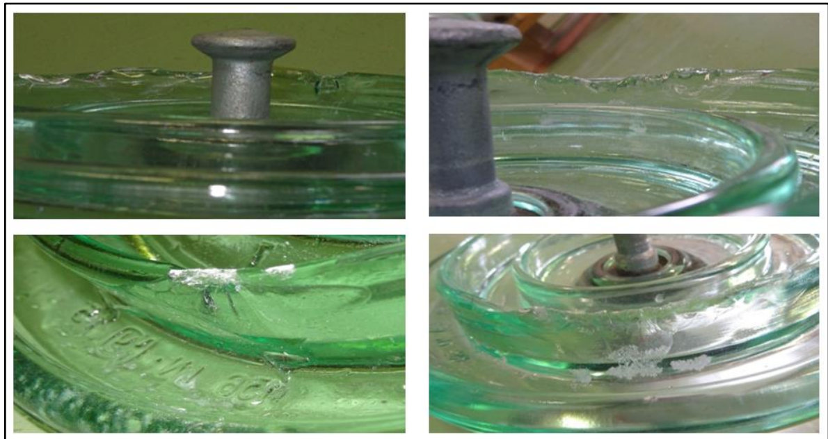
Figure 5 : low quality glass with bad toughening: no shattering while damaged
