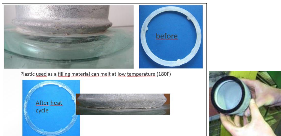
Figure 10: thermal degradation of plastic rings at the base of the cap (picture at right shows a cap with “flock” applied at the base of the cap prior to being assembled).
