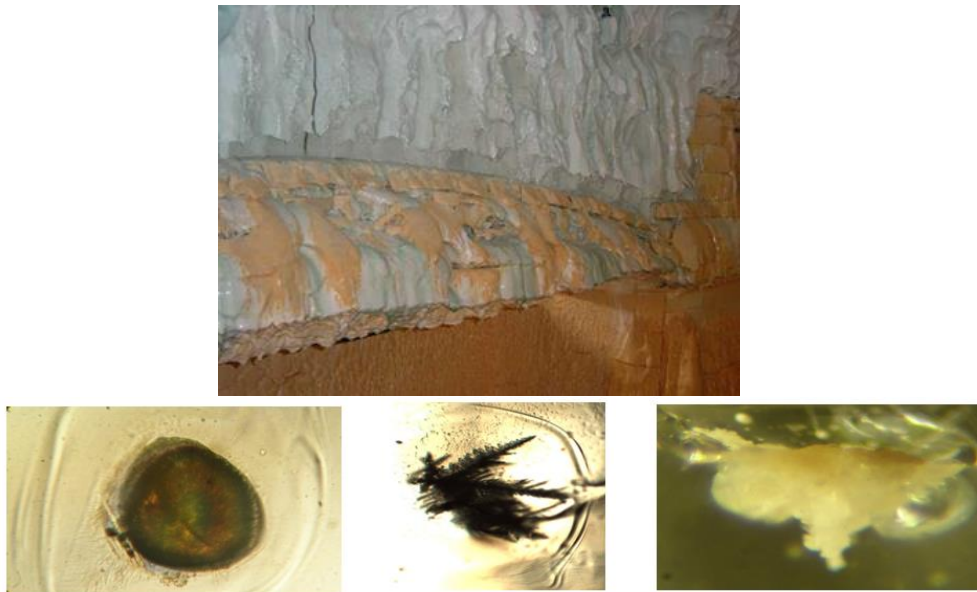
Figure 1: inside of a furnace after several years of operation: refractories are eroded (top). Examples of typical impurities found in glass (bottom)
