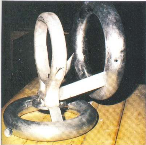
Fig. 16: Tube support for the endpoint: the vertical ring shields the end of the busbar (high risk of corona discharge), the horizontal ring protects the shielding of the insulator head.
