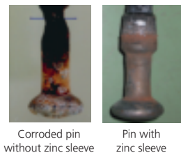
Pins from service insulators
